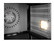
**Catalytic Liners** Reversible catalytic liners absorb grease residue from cooking. At high temperatures the grease is converted into ash and can then be simply wiped away.
