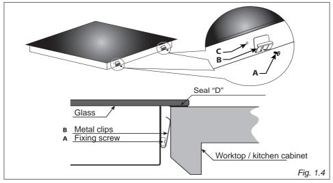
IMPORTANT: Spread the sealing material "D" around the edge of the hob (edge of the glass). The sealing material "D" must be installed correctly to guarantee a perfect seal between the appliance and the unit. Incorrect installation may cause irreparable damage to the appliance.
